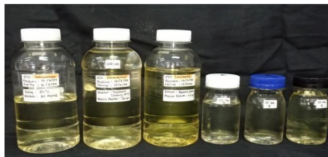
Figure 2. Results of the third method of VCO after filtration. A) Heating VCO, B) Fermentation of VCO, C) Enzymatic VCO.
